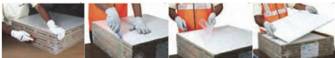
Wrong box opening method
